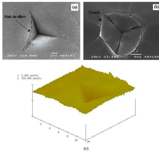
**Figure 5: SEM images of sample S1-6 at indentation depth (a) 500 nm (b) 1,500 nm and (c) AFM image of imprinted nano-indentation at 700 nm.**
