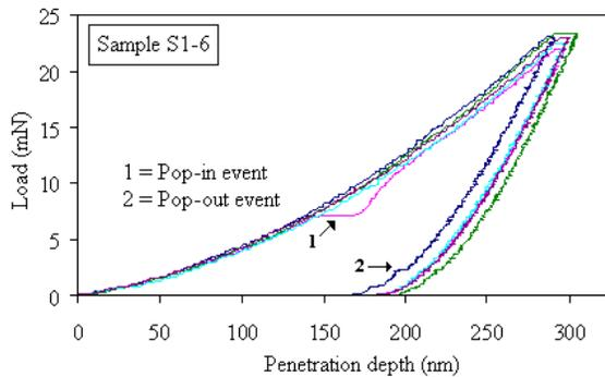
**Figure 4: Load-displacement curves of sample S1-6.**
