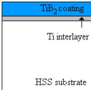
Figure 1: Schematic of single layer  $TiB_2$  coating on HSS with a Ti interlayer.
