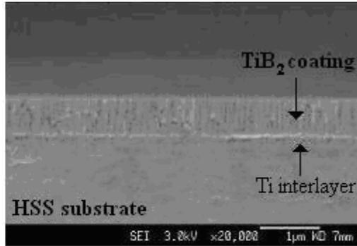
Figure 2: FESEM image of fractured cross-section of samples S1-6.
