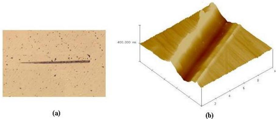
**Figure 6: Microscratch tracks measured by optical microscope (a) and AFM (b).**
