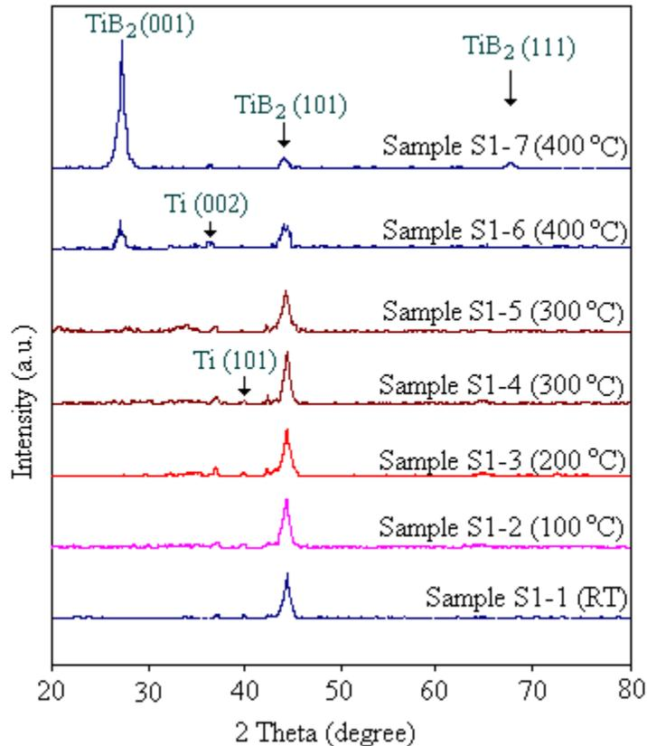
**Figure 3: XRD patterns generated from single layer TiB<sub>2</sub> coatings with a Ti interlayer.**
